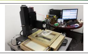
The Confocal 3-Axis Metrology System raster scans using a 3-axis motorized platform, built on a low-vibration granite base for optimal Confocal point sensor resolution and high quality 2D & 3D data visualizations for measurement & inspection applications.
